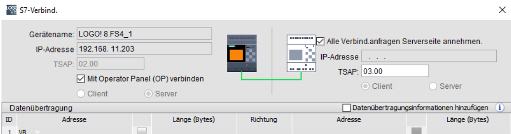
Image 5: Configuration of LOGO! connection settings. The same applies to a S7-200.
